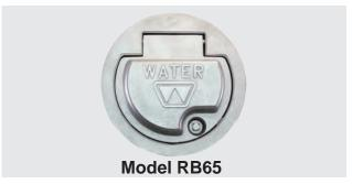
Exterior Finish: Box & Door - Chrome (CH) Only Designed especially for tilt-up wall construction. Install through 6" diameter hole. Two 3/8"-16 tapped holes for all-thread anchors in back of box. Lift and latch door stays open when hydrant is in use.
