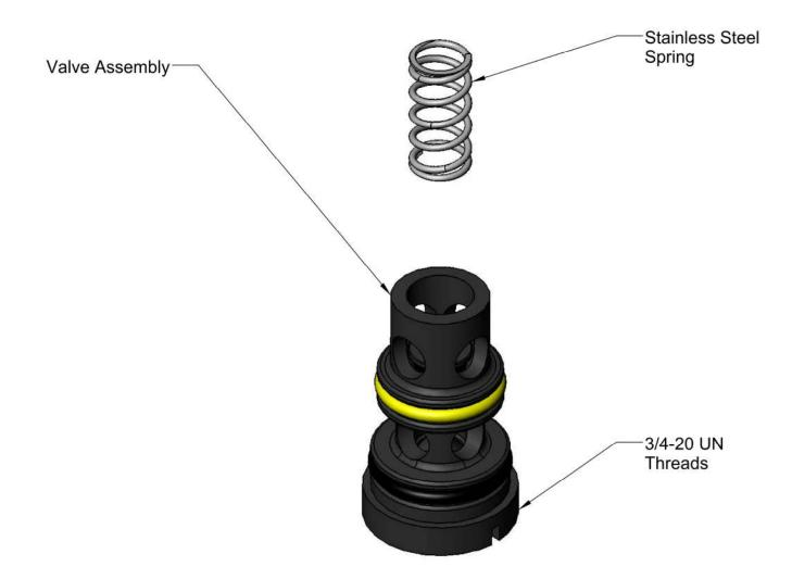
Checked Drawn Approved Product Specifications: **JRM DMH JHB** Valve Assembly Date: Scale: 2:1 12/19/08
