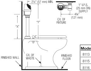
Model 8115 & 8116 valves are designed for installations where the water supply is roughed-in 24" - 27" (610 mm - 686 mm) above the top of the water closet.
