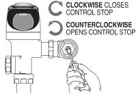
Adjust Control Stop after each flush until the rate of flow delivered properly cleanses the fixture.
