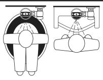
3. When the user steps away, the loss of reflected light initiates an electrical "one-time" signal that activates the flushing cycle to flush the fixture (1 second for urinal, 3 seconds for closet). The Circuit automatically resets and is ready for the next user.
