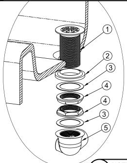
3 Install grid strainer and close elbow to bowl using plumber's putty.
