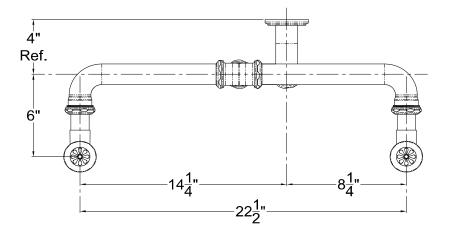
Assemble continuous waste piping using Teflon tape on all threaded connections and make up waste connections to 1-1/2" P-Trap.
